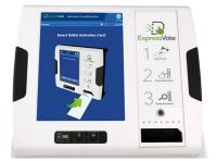
Pictured above is the Ballot Marking Device. A blank ballot is inserted into it, you make your selections, and your voted ballot is printed out. You then place your voted ballot into the ballot box.
